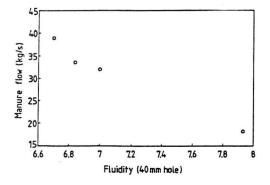
Fig. 9. The relationship between fluidity and the 'constant level manure flow' obtained when unloading an Omas vacuum tanker.
