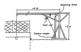
Fig. 2. The ball method. The hollow steel ball ( $\emptyset$ 82 mm) is filled up with lead pellets to a bulk density of slightly more than 7 kg/dm<sup>3</sup>. Using three different counter-weights, the ball can be counterbalanced to reach net weights corresponding to the bulk densities 3, 5 and 7 kg/dm<sup>3</sup>.
