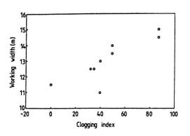
Fig. 10. The relationship between clogging index and the working width of an oscillating spout broadcaster attached to an Omas vacuum tanker.
