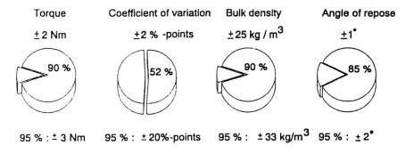
Fig. 13. Measuring accuracy when characterizing non-pumpable manure filling the box three times compared to five times. The calculations are based on data from six farms, giving rise to, as a total, 60 box combinations.
