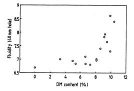
Fig. 6. The relationship between fluidity (measured with the 40 mm hole) and the DM content.
