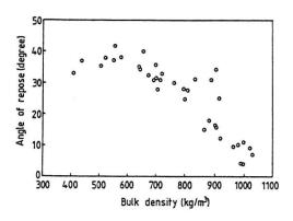
Fig. 12. The relationship between bulk density and the active angle of repose.
