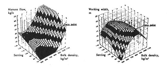
Fig. 14. The relationship between bulk density, setting and 'constant level manure flow' for a Kidd Tankaspread 1500.
