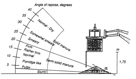
Fig. 11. The active angle of repose as measured with the characterization box for different types of manure.
