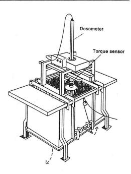
Fig. 5. The characterization box for non-pumpable manure. The box holds  $1.3 \text{ m}^3$  of manure and weighs 480 kg with and 300 kg without the lifting stand. The desometer plate is 250 mm in diameter and has six 100 mm long spikes underneath.
