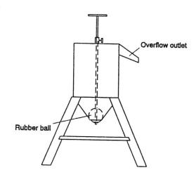
Fig. 1. The fluidimeter developed at JTI. The volume is 15.5 l and the outlet hole  $\emptyset$ 50 mm. The hole can be easily changed to  $\emptyset$ 40 mm using an additional cone.
